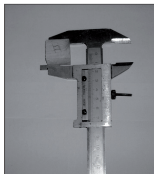
Fig. 7. A calliper, accuracy class 2.
