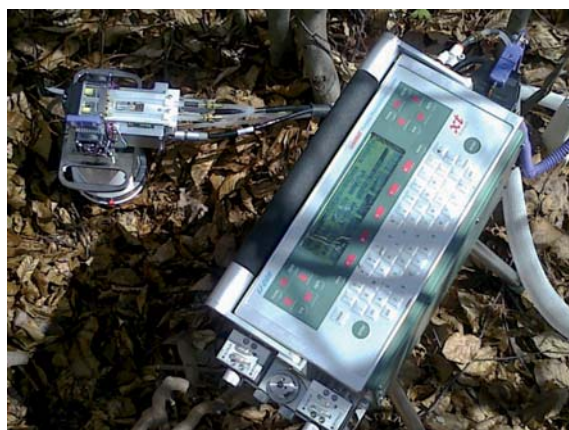
Fig. 1. Details of portable photosynthesis system Li 6400XT with a 6400-09 soil CO 2 flux chamber (left) and soil collar (right)
